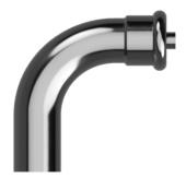
The fittings and tube shall be drawn from the Eco Duo Copper Press fittings (available from Water Kinetics), manufactured from copper with EPDM 'O' rings. These fittings are for jointing copper tube and are available in sizes 15mm to 108mm. The fittings shall incorporate a "leak before press" facility offering a final check of the system to provide instant identification of joints that are assembled correctly but left unpressed. The fittings shall also offer electrical continuity.
