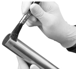
5. If silver brazing alloy is being used, apply flux to the outside of the tube where fitting will be brazed. If a copper/phosphorus alloy is used, no flux is needed.
