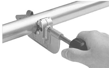
2. To cut the inner tube, slide it out from outer to expose it for cutting. Cut the tube as you did for the outer.
