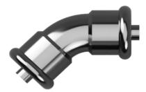
The fittings and tube shall be drawn from the Eco Duo Copper Press fittings (available from Water Kinetics), manufactured from copper with EPDM 'O' rings. These fittings are for jointing copper tube and are available in sizes 15mm to 108mm. The fittings shall incorporate a "leak before press" facility offering a final check of the system to provide instant identification of joints that are assembled correctly but left unpressed. The fittings shall also offer electrical continuity.
