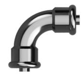
The fittings and tube shall be drawn from the Eco Duo Copper Press fittings (available from Water Kinetics), manufactured from copper with EPDM 'O' rings. These fittings are for jointing copper tube and are available in sizes 15mm to 108mm. The fittings shall incorporate a "leak before press" facility offering a final check of the system to provide instant identification of joints that are assembled correctly but left unpressed. The fittings shall also offer electrical continuity.
